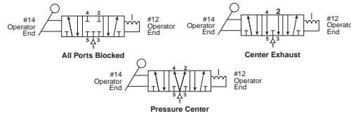
*Single pressure at Port #1* – The Hand Lever alternately pressurizes port 2 or 4 while exhausting at port 3 or 5.
