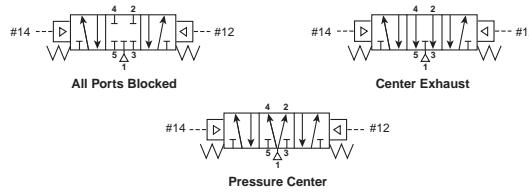
*With #12 operator signaled* – inlet port 1 connected to cylinder port 2, cylinder port 4 connected to exhaust port 5.
