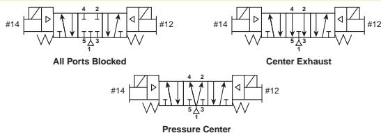
*With #12 operator energized* – inlet port 1 connected to cylinder port 2, cylinder port 4 connected to exhaust port 5.
