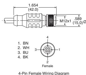
4-Pin Female Wiring Diagram
